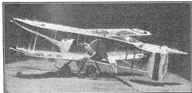
Since the "Gun Bus" is a pusher rather than a tractor, the prop and engine—as can be seen—are mounted to the rear of the fuselage. The wing and tail insignia on the model are optional, since the earlier planes were seldom marked.
