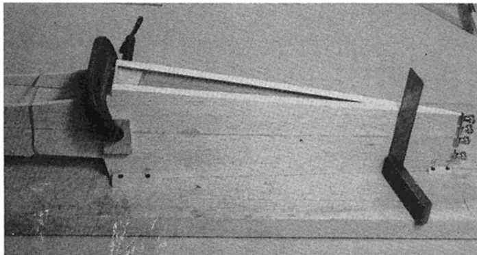
Tailpost being glued in. Note fixtures to hold fuselage sides in place while glue dries. Also use of square to check fuselage sides.
