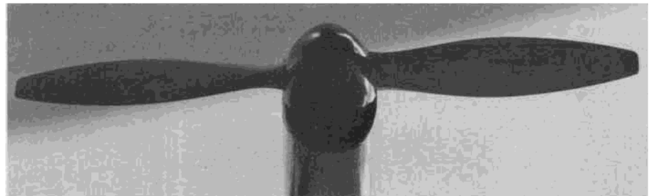
Business end features a non-folding Rev-Up prop (11 x 7-3/4), spinner, Leisure Electronics 05 motor with gear box, and air scoop to cool motor.
