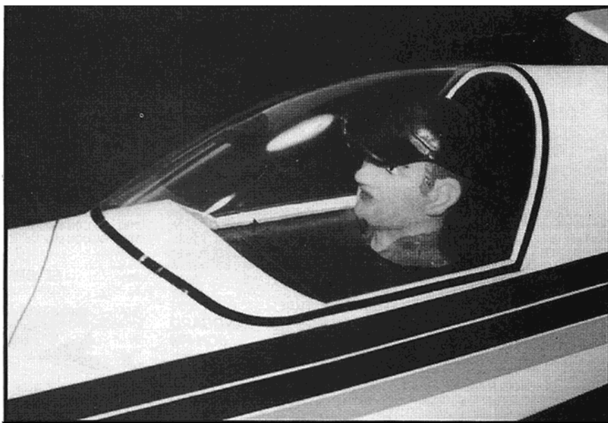
Ace R/C Canopy is neatly adhered with RC56 Glue and Multi Stripe Tape. Pilot figure is part of D.G.A. 1/4 scale pilot bust kit, painted with model car enamel.
