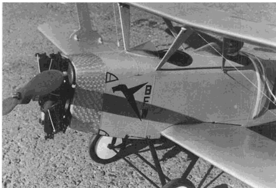
The author used Williams Bros. Le Rhone cylinders to duplicate the Siemens radial on the full-size aircraft. That prop is strictly for display and was put on for these photos (that's why there's no AMA safety nut). Udet's flying scarf is about due for a replacement, we think.
