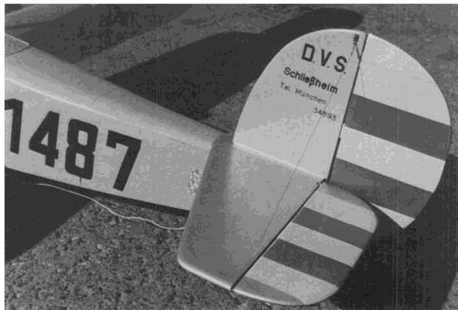
Large numbers on wings and fuselage were masked off and sprayed with Aerogloss dope, while smaller markings such as those on the fin are done with rub-off transfers from art supply stores.
