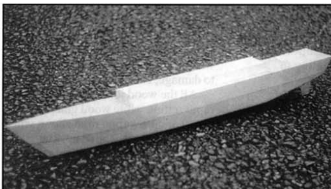
LEFT: The superstructure is built over the 1/16" plywood deck coaming. RIGHT: Close-up of the bridge and fore funnel.
