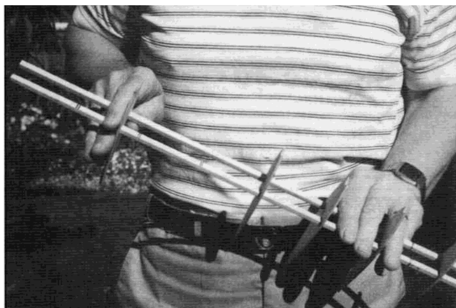
Sliding the ribs onto the spars.
