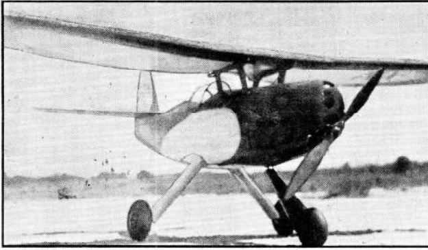
The nose wheel protects the propeller in bad landings
