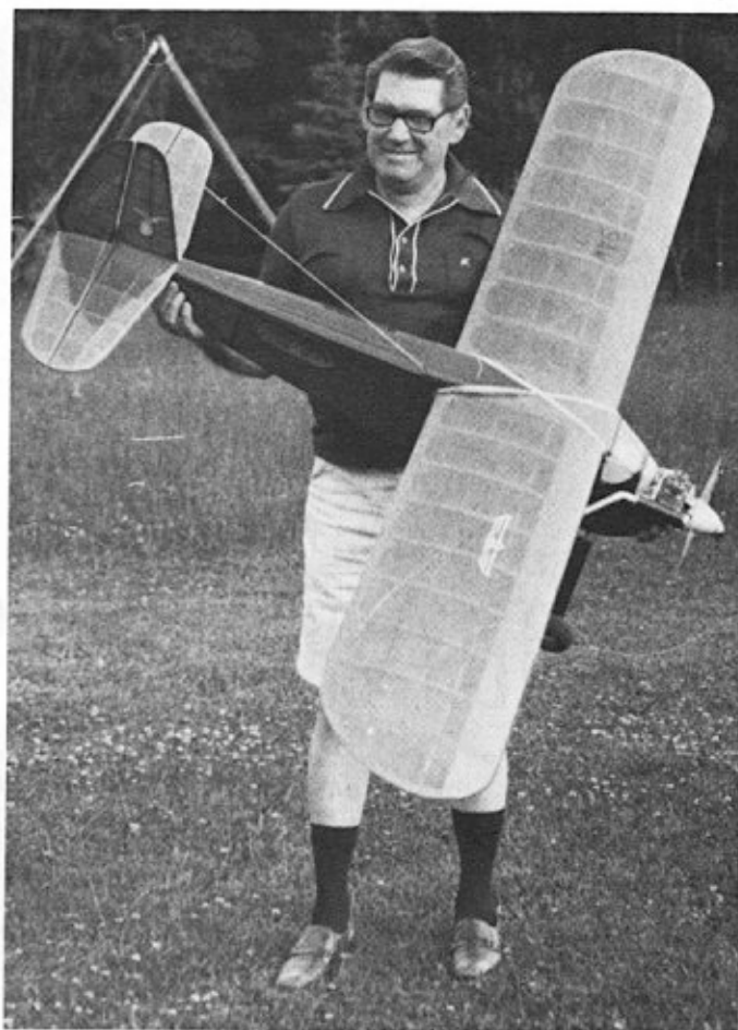
George shows the topside of TORC. Long tail moment assures stability.
