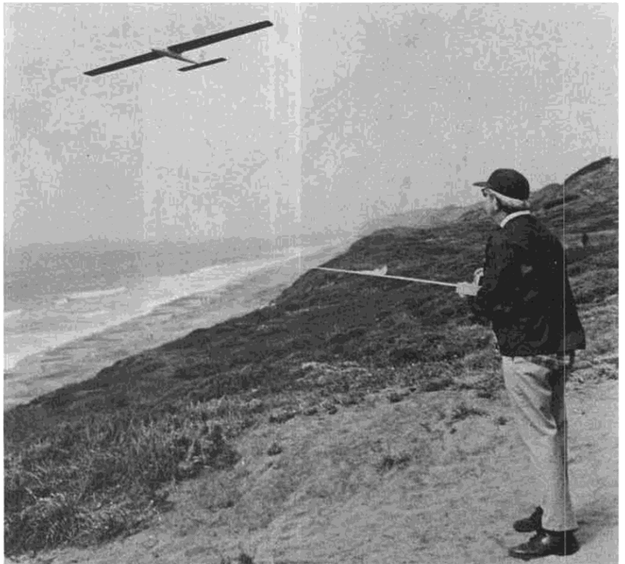
With nose slightly up, the Top Slider makes a relatively slow fly-by, Ken at the controls. The apparent droop of the wings results from the swept leading edge and minimum dihedral.
