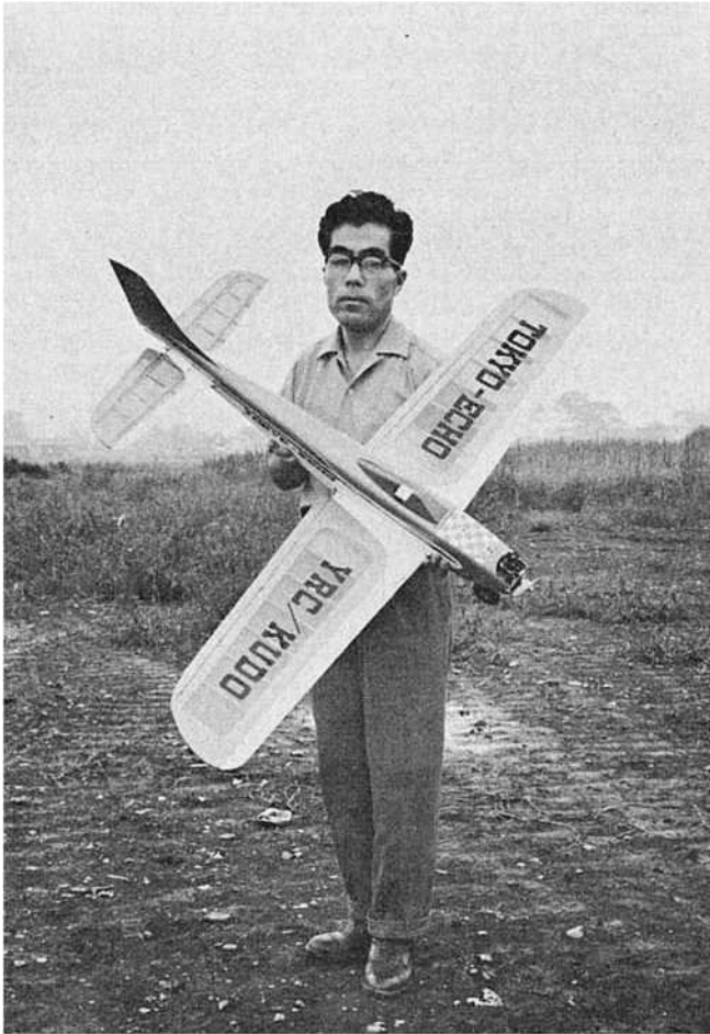
The author and a Tokyo Echo prototype. A new standard in single channel performance with aileron-only control. Has been flown 6-channel with slight modification.
