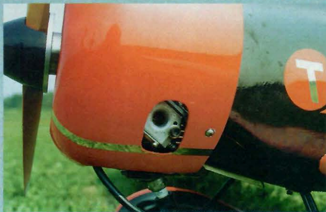
The size of the cowl easily fits the Zenoah and its muffler, but John opened a hole for access to the carburetor (above left). He can choke the engine more
