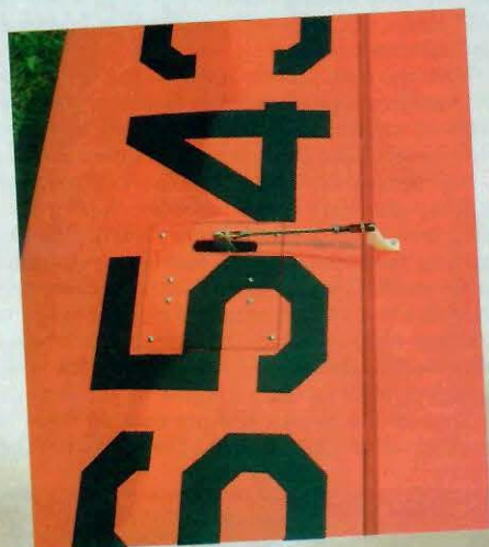
There's a servo in the bottom of each wing to drive the ailerons. They nest in a servo bay with a hatch. Screws in the four corners hold the hatch. The other four screws hold the servo mount.
