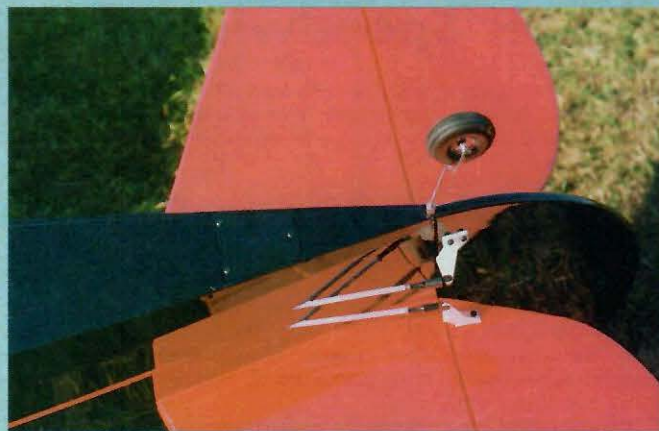
readily for starting. Control setup is pretty conventional (above right), but be sure to use stiff strong pushrods. Use a good strong tailwheel unit also.
