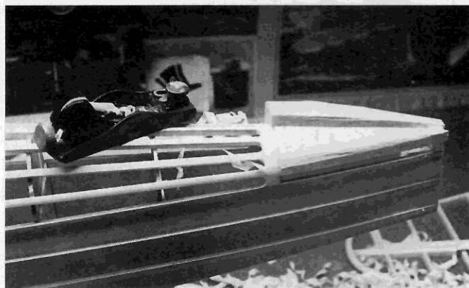
before final sanding. The bows of the tail group were formed around a template from a laminate of four strips of \frac{3}{32} \times \frac{3}{8} inch balsa (below left). After the inner framework was added, the control surfaces are ready to be cut out (below right).
