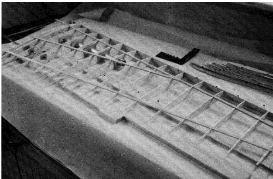
The wing is built upside down over the plans, so that the top surface will be straight, with no dihedral. Trailing edge of ribs shimmed to ensure a straight and true structure.
