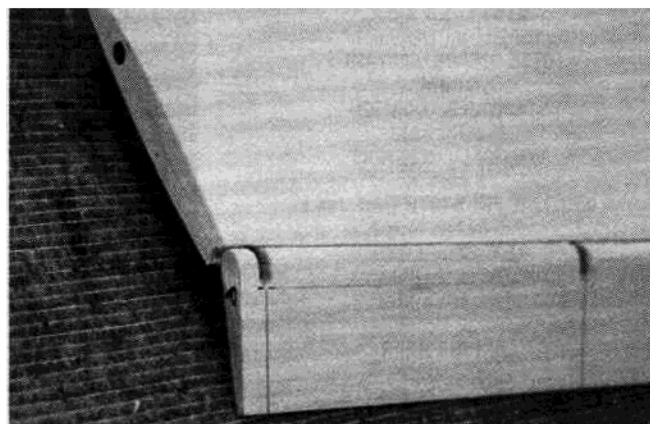
LEFT: Aileron set-up showing the effect of the offset hinges (up aileron shown). RIGHT: Aileron down. Take your time and get a good fit.
