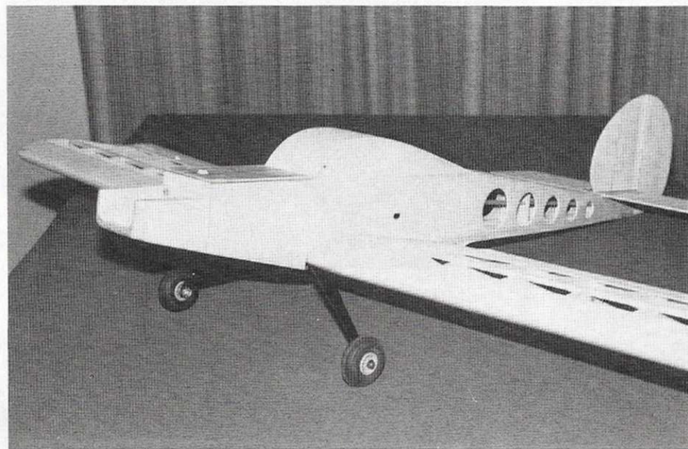
The completed framework shows the lightening holes in the fuselage sides. They're made of poplar ply and require no additional doubling. However, as a precaution, the author added bracing to the tail.
