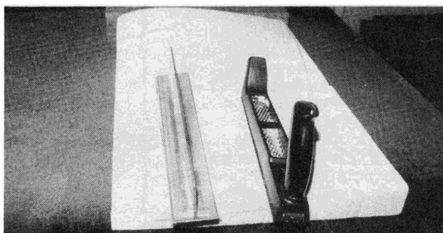
With the bottom wing skin glued in place, the tip template is placed in position, and the top shape of the wing is formed using coarse sandpaper, or other tools like the Stanley Surform.
