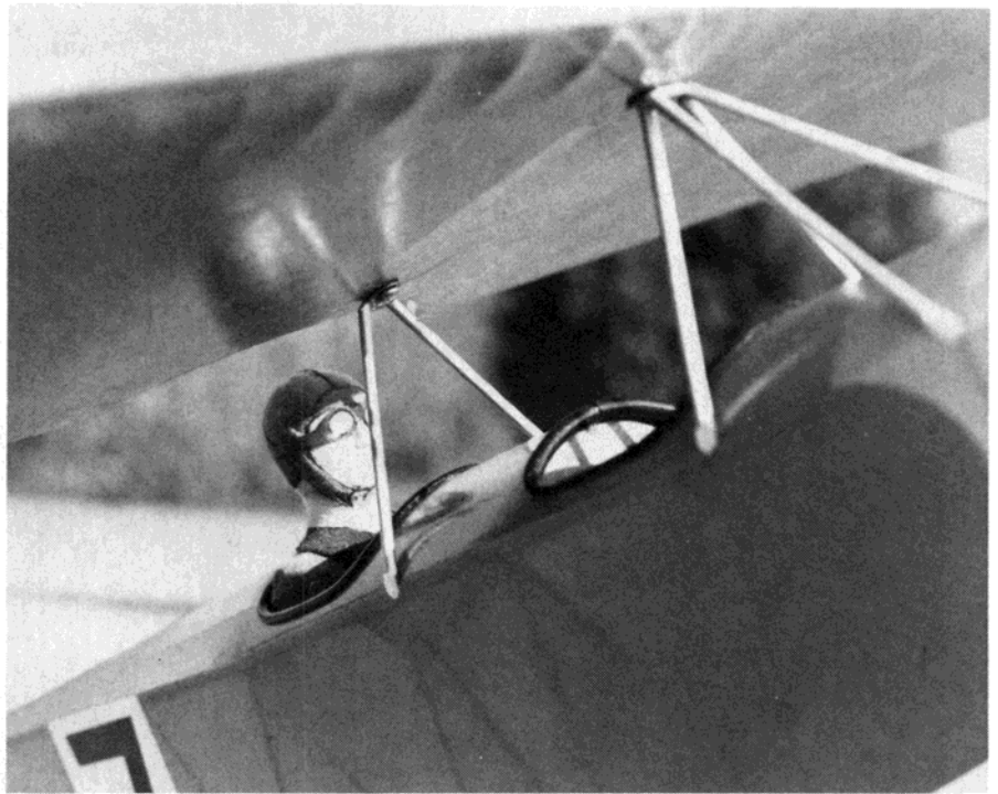
Two or three channels guide the 1/2A Sparrow II by Don Snull ( at left ). To simplify final finish and covering, Don builds aluminum tubes into the fuselage to receive plug-in wires such as the cabanes ( above ).
