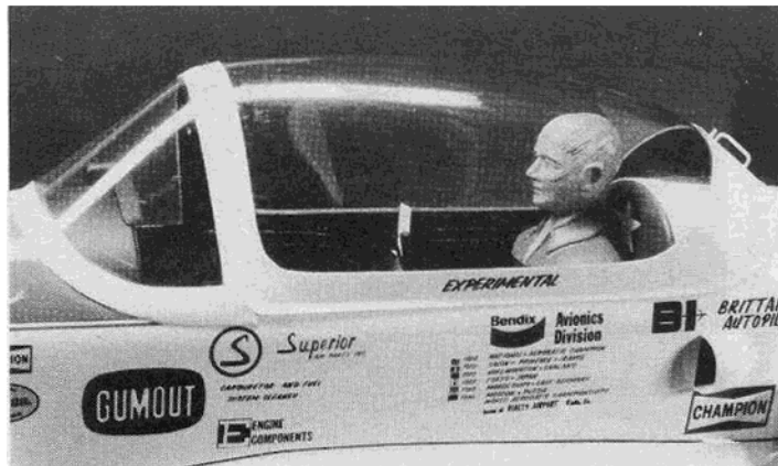
Finished cockpit with fiberglass canopy frame over clear plastic canopy. Modify Williams Bros. pilot to look like Art Scholl by changing hair, cheekbones and add mustache.
