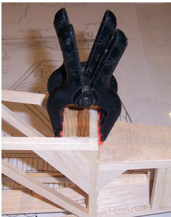
Tail skid spruce blocks glued into place.
