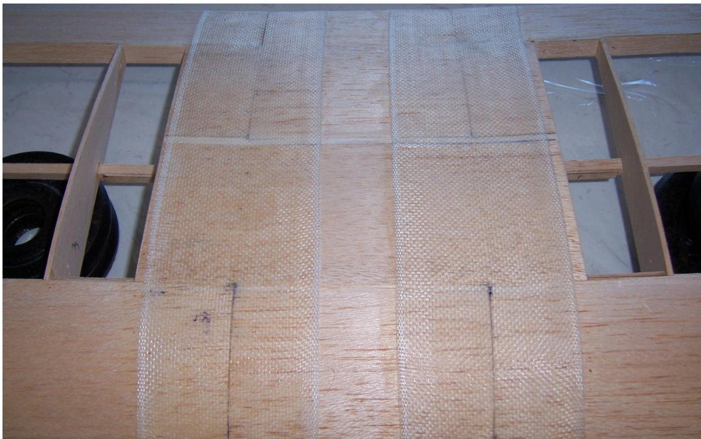
Wing join reinforcement bandages – 3" PVA soaked glass tape .These also provide protection against wing bands.
