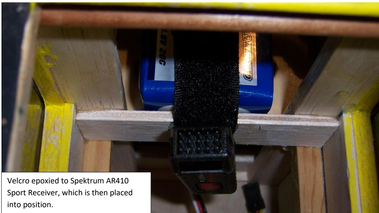
Velcro battery retaining straps epoxied into position.
