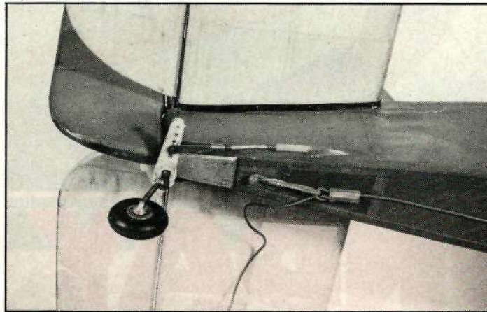
O.S. 20 four-stroke engine fits neatly into the cowl, note the remote plug and socket connection for the glo plug. Steerable tailwheel/rudder connection - plus tail weight for balance shown on left.
