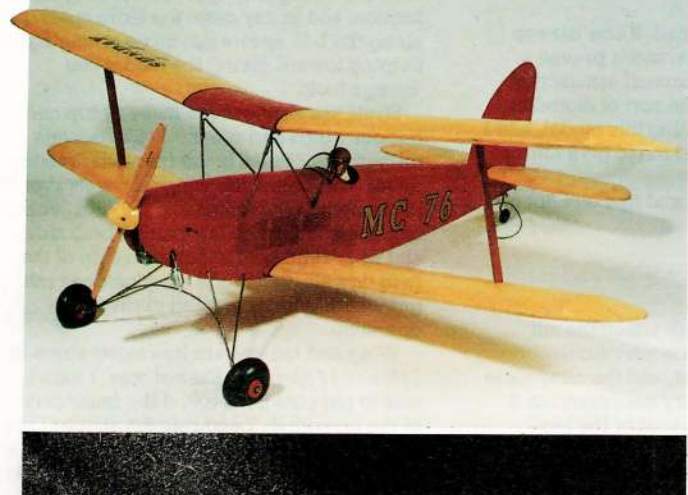
A very durable and practical design, the flying characteristics are the total antithesis of the 'Jean Machine' (also featured this month) as it is slow, stable and predictable - a true 'Sunday Flyer'. Covered in vintage style coloured Solartex the atmosphere of Mike's model is strongly reminiscent of free flight designs from the 1950's. No doubt the 'Sunday Flyer' could be converted to free flight operation - making a pleasant reversal of the normal trend!
