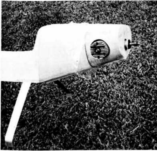
Ship is balsa and ply construction throughout. Only a few weeks old, and a trophy winner already. Akro placed second in scale at Corpus Christi Even cheek cowls are formed of 1/64 plywood. Internats contest, was judged by well known scaler. Tom Dean.
