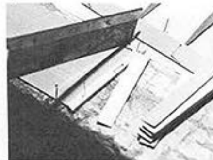
Simple jig using a stop of 3/32-inch scrap balsa, two guide pins and a razor saw to cut the shear webs.
