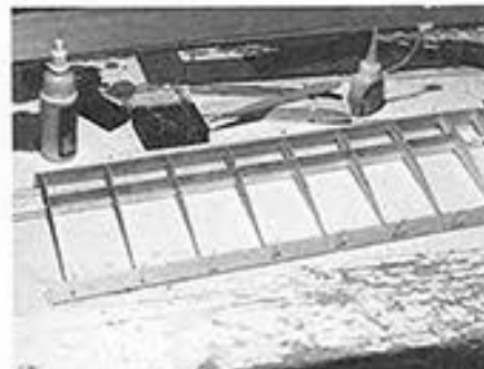
Detail of lamination of rudder outline. The technique is similar to that of the wing tips.
