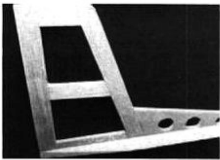
The vertical and dorsal fins are made as an assembly. Pin the assembly in place on the fuselage top and trim the rear of the fairing to match the fuselage.
