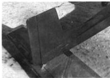
Finished but before trimming view of the tail. The rudder push rod exits on the left side similar to the horizontal stab rod shown.
