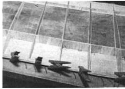
The bottom sheeting is dampened with water and rolled up under the leading edge. Titebond does the gluing job well. Clothespins (by the dozen) hold the bottom while glue dries.
