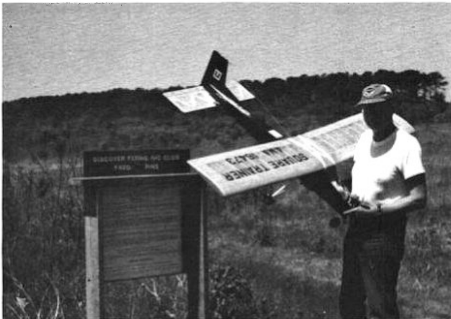
The author with his Square Trainer . You'd be hard-pressed to find an easier to fly first R/C model: high wing, tricycle gear and a forgiving airfoil. Building one is a good education too.
