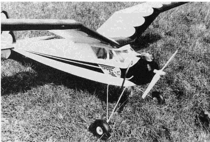
Spook showing 4-stroke tank location, copper exhaust pipe, Laser 60 engine, and Spook insignia.
