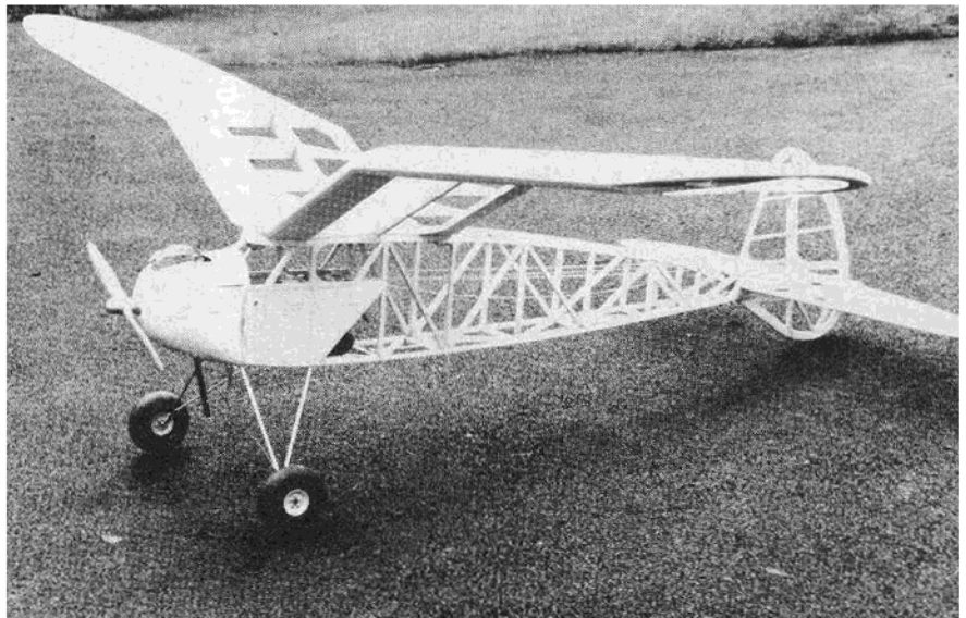
Detachable tail showing dacron control lines and plastic exit tubes glued in place.
