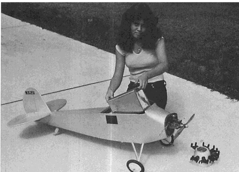
The R/C is all but lost within the cavernous interior, Cables to the rudder and elevator work well. Radio should be full forward if a large tank is ever contemplated. Left: Nancy McGovern shows how a standard gallon tank fits.
