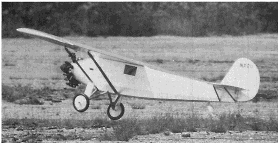
First take-off. A short run and that Clark Y lifting section does the rest. Tail surfaces are enlarged enough to make it mild of manner. Lower photo: Balance it at 25%. More new ships are wiped out because of lead-like tails than fingers can count. No ballast in nose was required, just shift the radio about.
