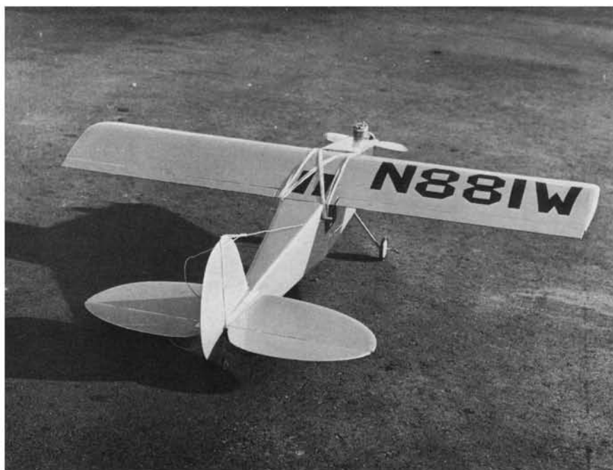
The Spirit of St. Louis can be "cleaned up" by using nylon wing hold bolts if you so desire.
