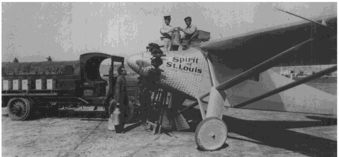
The "Spirit" getting refueled for one of its test flights at Rockwell Field, San Diego, California. Small sign under seat on side of truck says, "Standard Oil Company". Note solid truck tires with holes for "shock absorbing". Photo courtesy of Pete Westburg.
