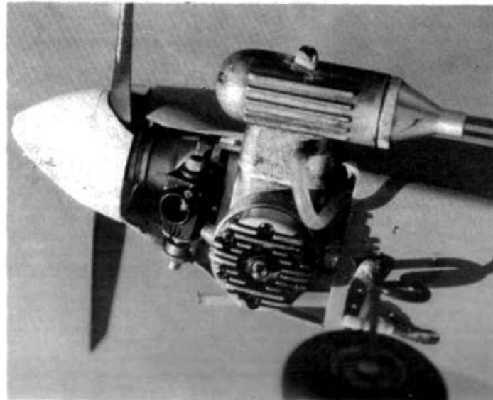
Below left: motor installation showing HB 25 used in original. Note external steering arm for noseleg. Below, right: Richard poses with the second prototype, and shows compact size of the model.
