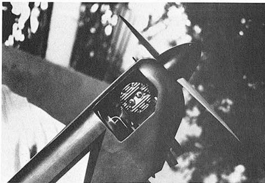
ABOVE: ST 71 is very comfortable in the spacious nose. The tank protrudes through the bulkhead for easy inspection. Tatone manifold ducts the goop out the bottom.
