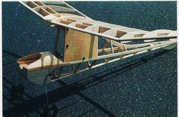
Radio access is by a removable 1/32" ply panel held in place with 4 plastic screws.
