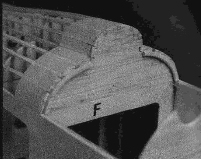
LEFT: Note cutouts for cooling in fire wall. RIGHT: Sheeting supports glued to front of Former F.
