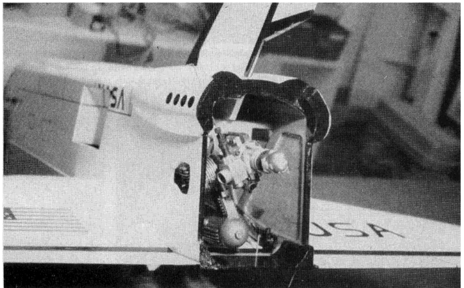
Engine and vertical fin installation.
