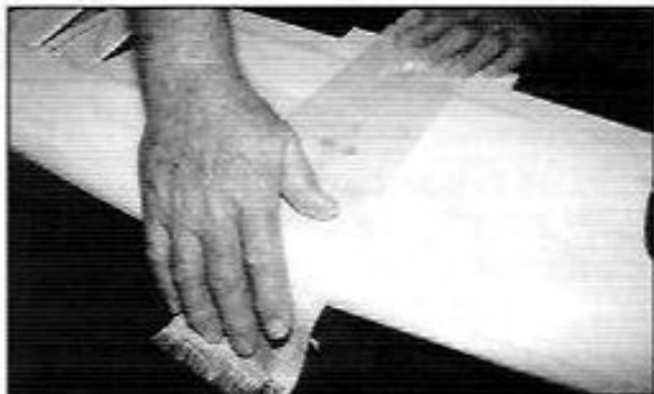
Southern Eagle uses a servo on each aileron. Note the holes cut for the servo pigtails to exit the top center section. The center section then gets glass and epoxy wrapped for strength.
