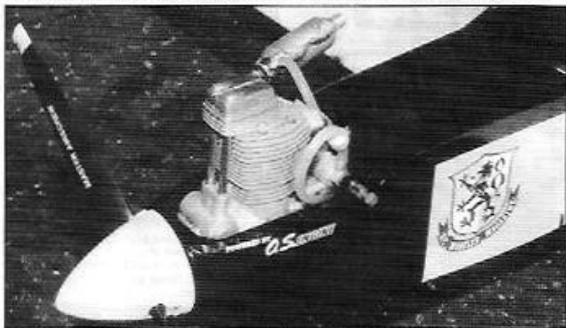
The .91 size 4-stroke is most popular, a 13 x 6 MAS prop and a 2-1/2" Du-Bro spinner.
