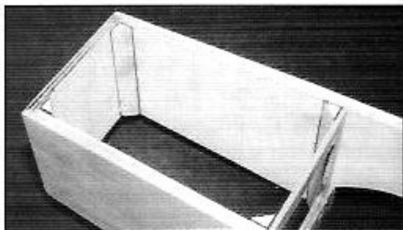
Note the use of triangular stock for strength.
