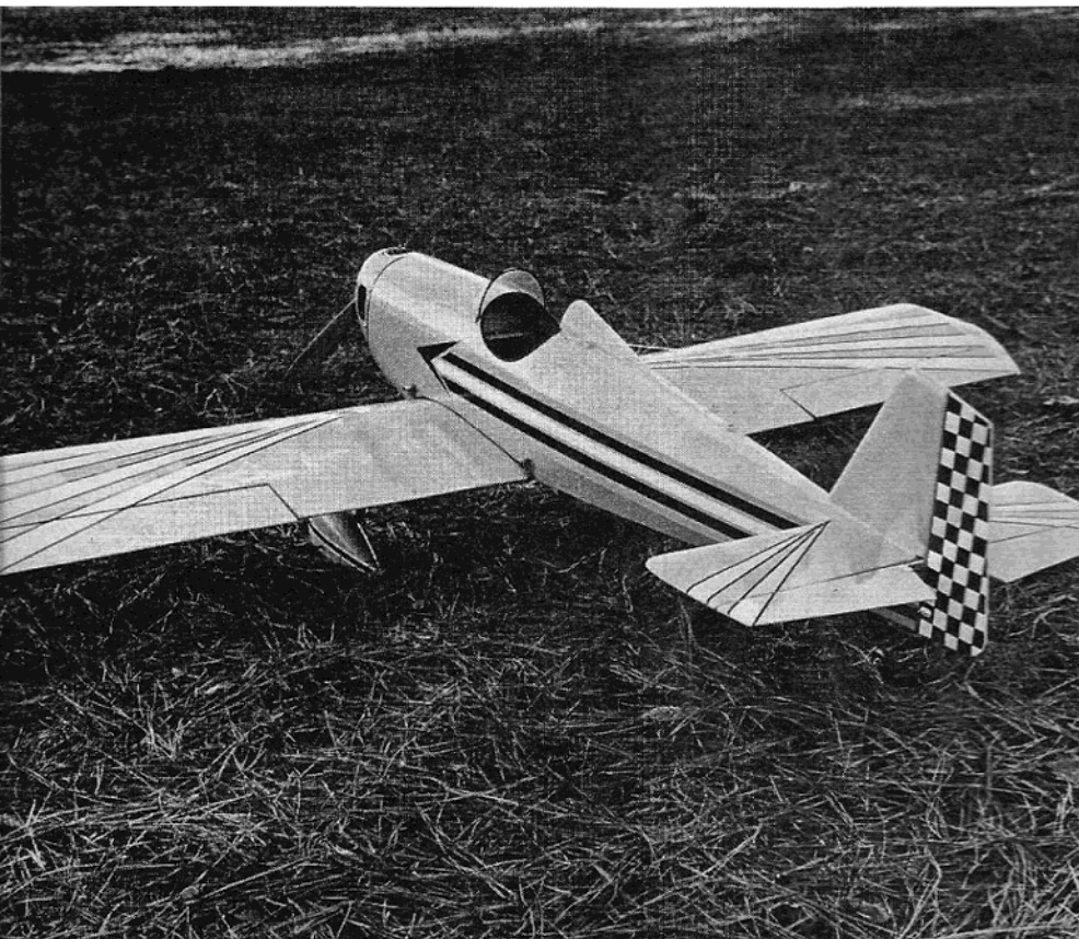
Blue MonoKote with black and white trim. Hire coolie to cut out checkers for you.
