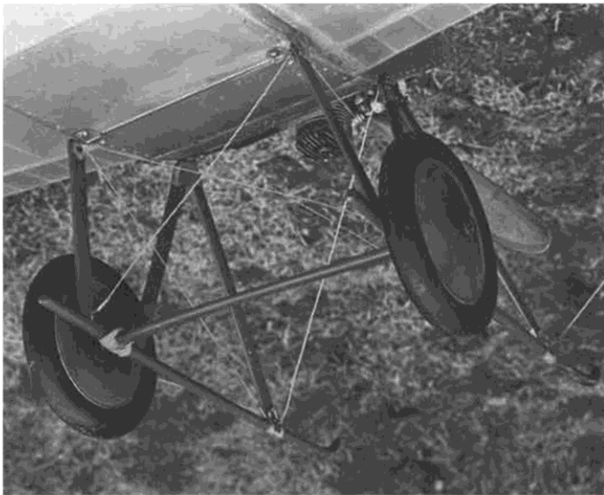
Detail photo of the undercart (this is a British plane, don'tja know) Note axle bound to skids with rubber. Williams Bros. wheels.
