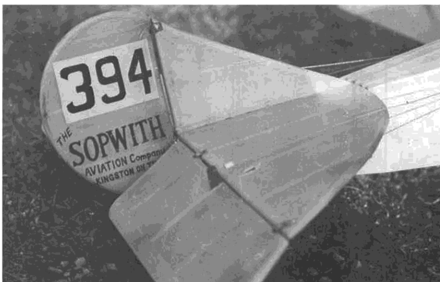
The sum total of the decoration on the Tabloid is right in this shot. Controls actually are operated by stranded steel cable. Curved outlines are laminated 1/32 balsa strips.
