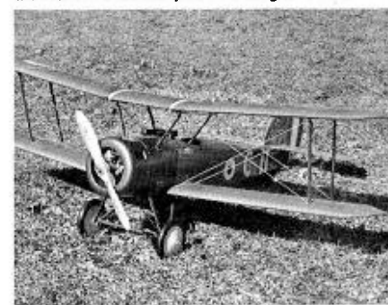
While author made a built-up balsa cowl, an aluminum kitchen pan also might work.
