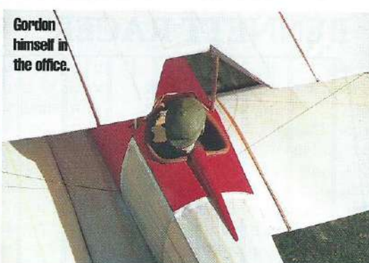
Completed fuselage awaiting final colour details. Rigging wires are installed.
