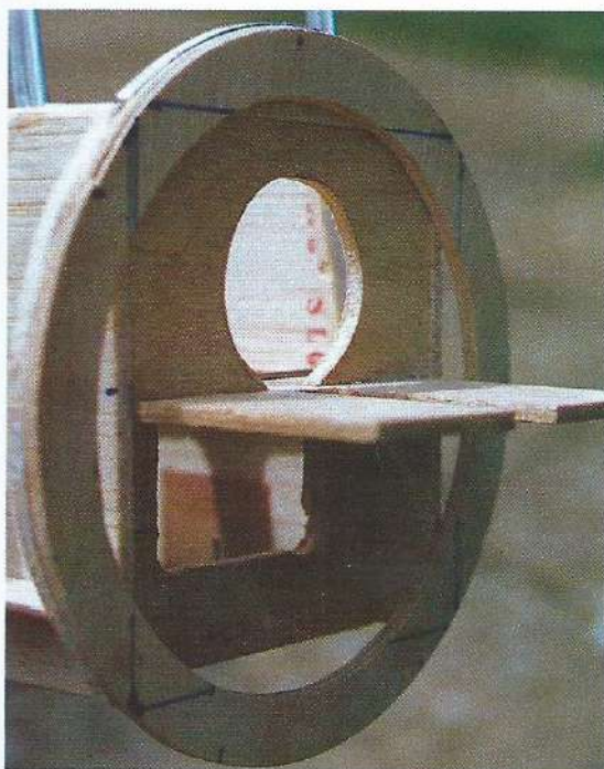
Below: motor bay showing the ply plate motor installation bearer and the false rings at the "firewall" that create the shape of the fuselage front end.
