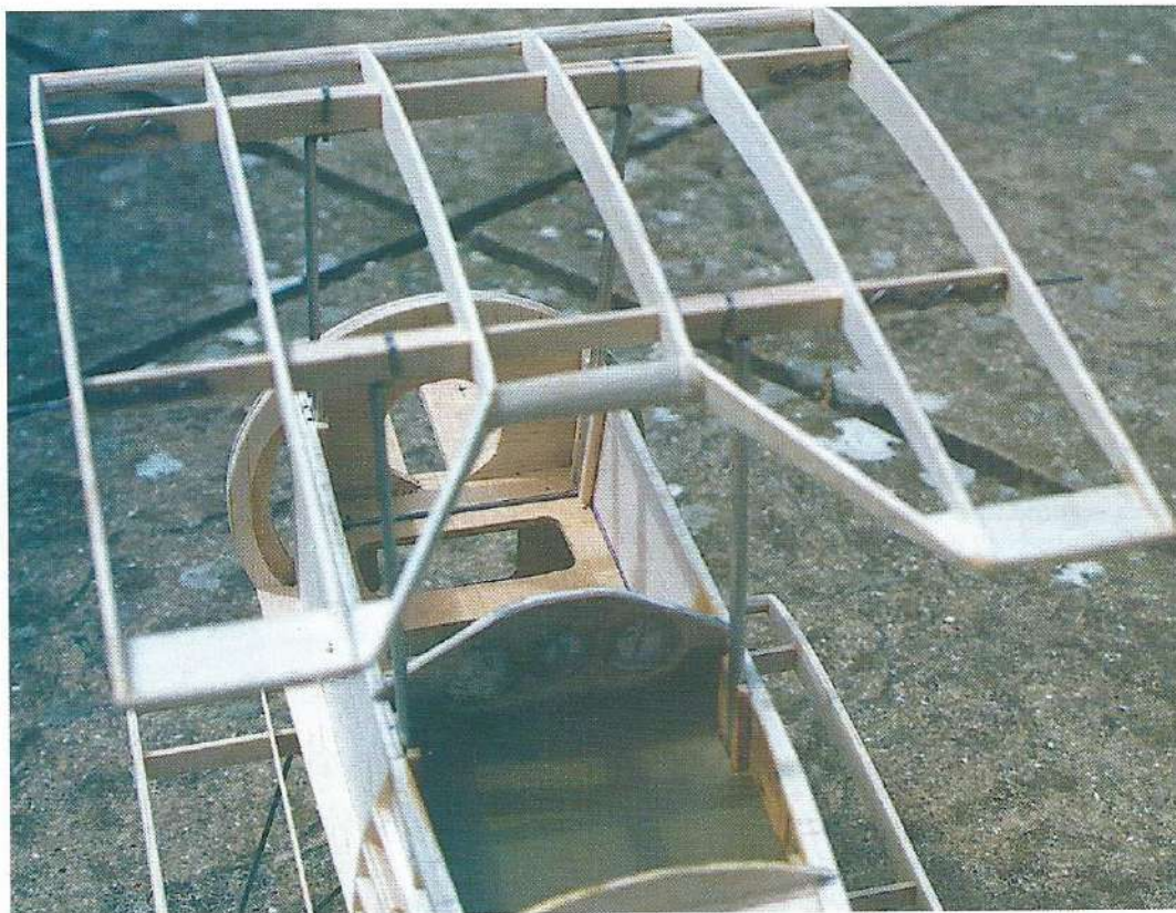
Above: Upper wing centre-section on cabane struts; Mike forms these from thin wire faired with carefully squashed alloy tube. Right: Cabane struts in close-up showing split-pin fixing method.
