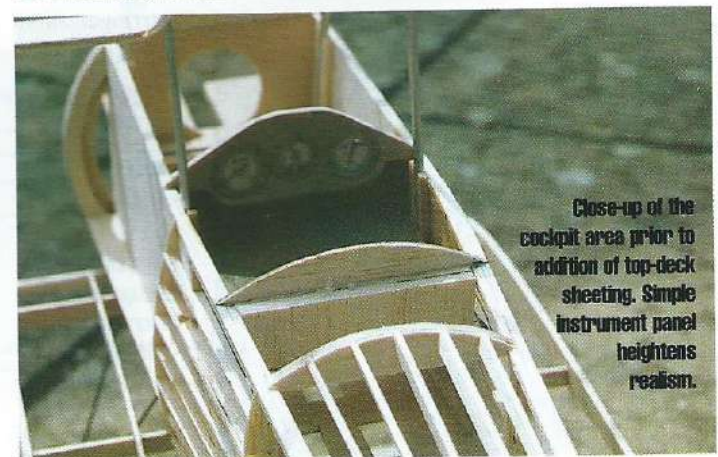
The multiple stringered rear fuselage.
