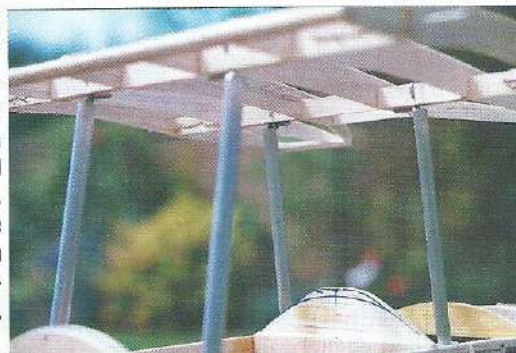
Above: Upper wing centre-section on cabane struts; Mike forms these from thin wire faired with carefully squashed alloy tube. Right: Cabane struts in close-up showing split-pin fixing method.
