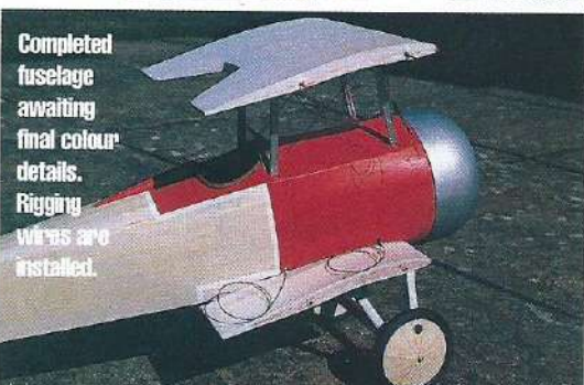
Engine cowl came courtesy of Caymer's Cider! Their three litre bottle is exactly the right diameter
