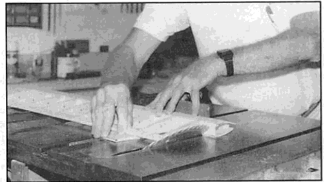
A table saw cuts off the wingtips neatly at 45°. Note shim under TE.
