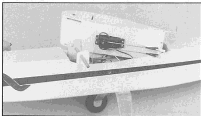
The wing center section with aileron servo normally remains in place for storage but can be removed by withdrawing the dowel.
