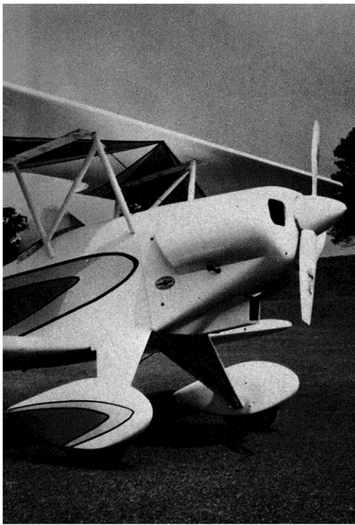
The 88" span biplane has 2,600 sq. in. of area, and comes out at a projected weight of 26 pounds. As with any biplane, the more cubic inches you can pack under the cowl, the better aerobatics will be.
