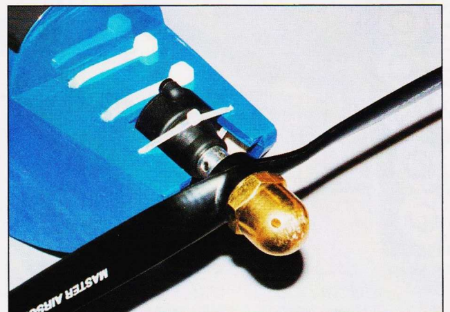
Close-up of the motor and Master Airscrew 3:1 gearbox mounted in place.
