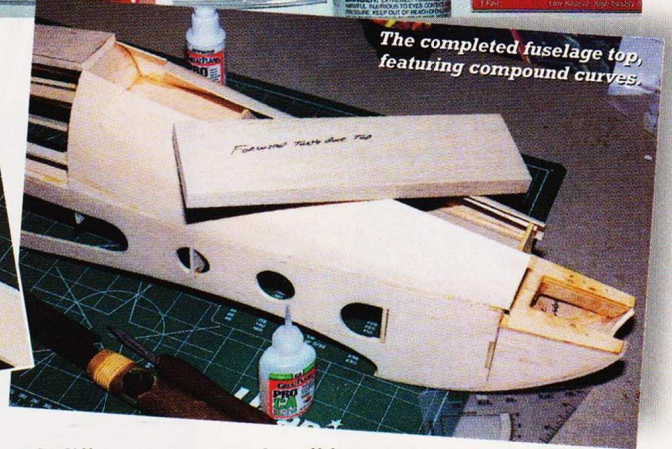
Rear turtle deck, ready for carving / sanding. Everything seems to fit perfectly.
