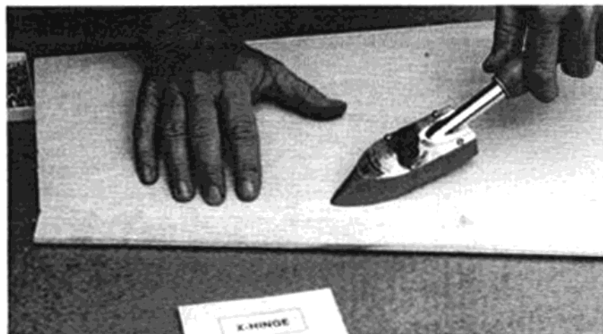
Pin control surface in place on wing, then Iron down X-hinge on to wing.
