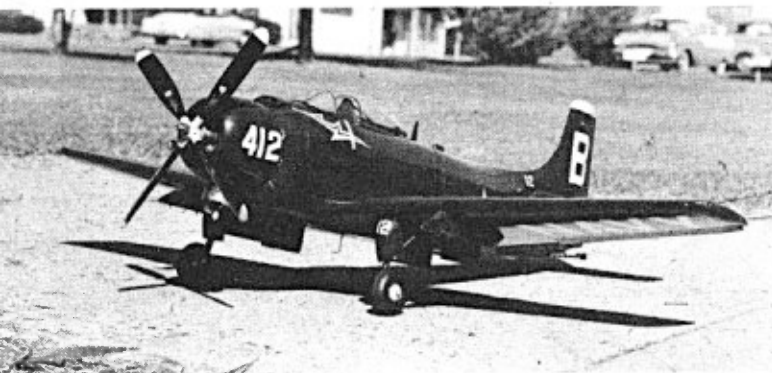
Only the exposed head of the inverted engine differs from true scale. Landing gear, for example, is most realistic, but is durable in use.
