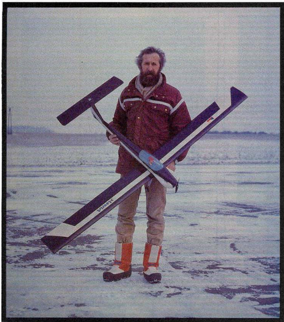
Designed by Pavel Bošak, this two meter powered glider makes an ideal way to get started. Designed for three function radio with a .10-.15 size glow for power. Could be set up for electric also.
