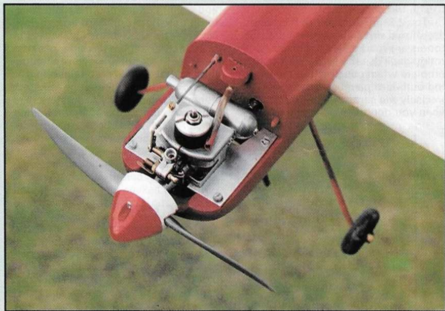
The aluminium engine mounting plate allows for quick and easy changes of the powerplant and is also a real boon when servicing the model.
