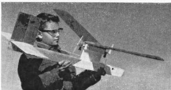
Cylinders separated! Push-pull twin .049 glow plug engines powered Mark III as a variation on the "Simpleton" theme—with radio control.
