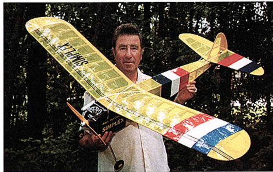
Stu used transparent yellow film on the top of the wing and slab, opaque dark blue on the bottom. Dark colors make for excellent in-flight visibility, especially at high altitudes.
