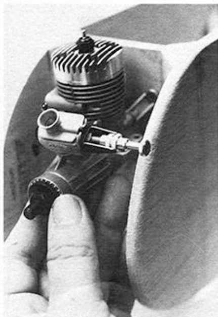
The K&B .20s spider mount works ideally. An aluminum or glass-filled nylon radial mount or hardwood beam mounts can be substituted for other engines.
