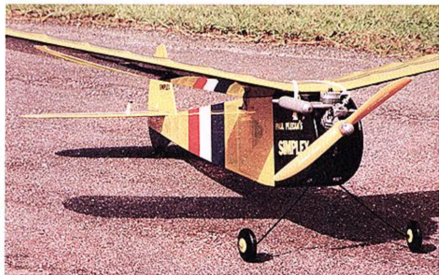
The 12x6 Antique series Master Air Screw prop parallels the shape of the old Flo-Torque props of the 1940s. K&B Sportster .20 turns this prop at 5000 rpm max, 1400 rpm idle.
