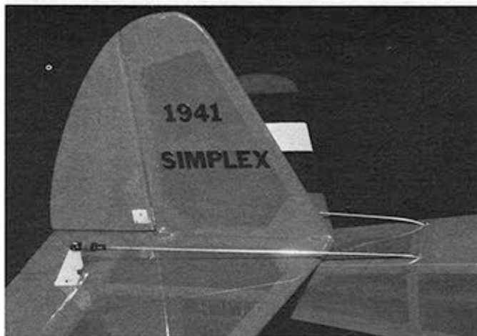
Flat tail surfaces go together fast and easy. Model has an elevator on just one side of the stab, works fine.
