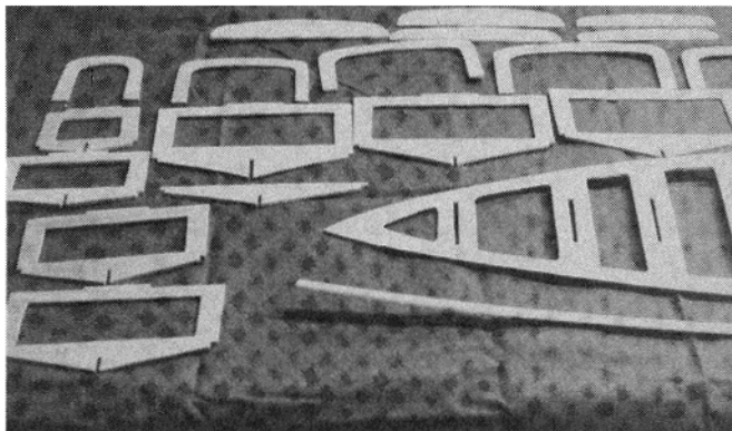
Hull crutch, keel, bulkheads, and formers ready for assembly.
