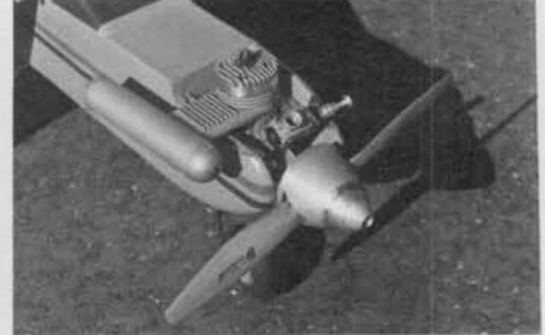
K&B Sportster .20 installation. Note muffler with adjustable exit port to push exhaust gases in any direction.
