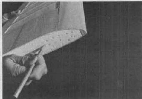
Use pencil to make holes in foam to improve bonding of wing halves. Note leading edge contour.
