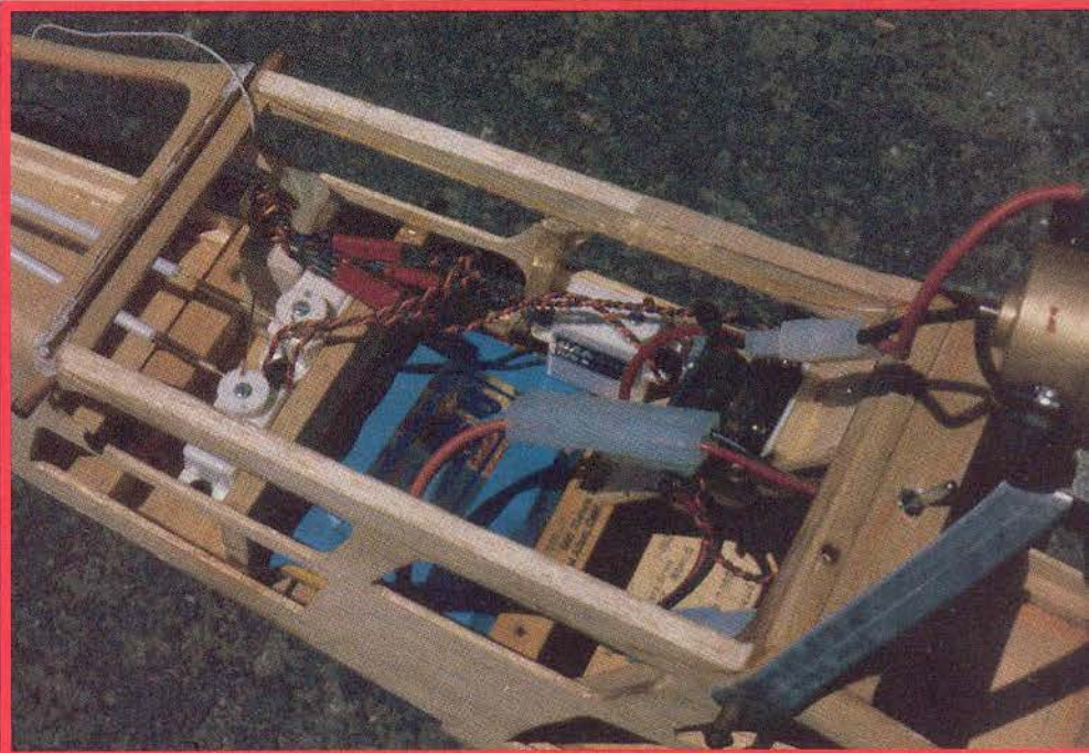
Equipment compartment — servos, receiver, micro-switch, motor batteries. (Motor batteries moved forward later for balance.)
