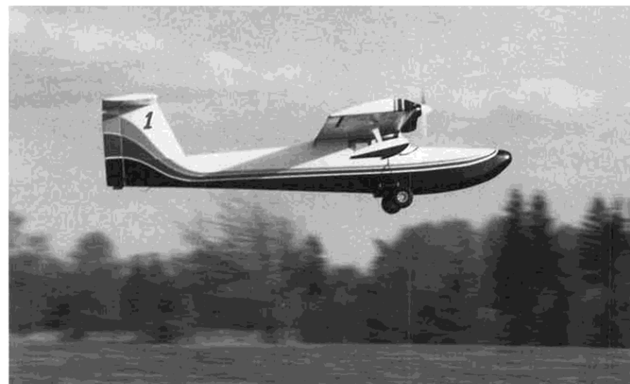
The prototype Seasport II is fitted with a removable landing gear for dry-land flying. This is detailed on the plan, but dyed-in-the-wool seaplane fliers may want to leave the gear off altogether.
